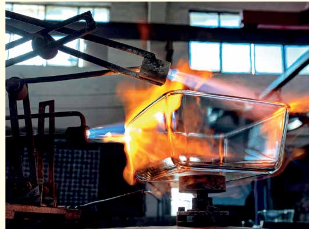
我們為一家位於山東省淄博市的玻璃廠供應天然氣，用於玻璃產品做模、拋光等工序。 We supply gas to a glass factory in Zibo, Shandong province for manufacturing processes such as forming and polishing.
