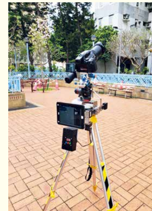
「全方位立管檢查」方案，提升檢測效率，並免卻僱員高空工作之風險。 The 360-degree Total Riser Solution improves inspection efficiency and eliminates the risk of employees working at height.
