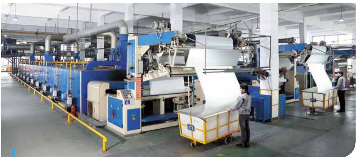
Stenter machines heated up by natural gas are used at a textile mill in Suzhou, Jiangsu province.
