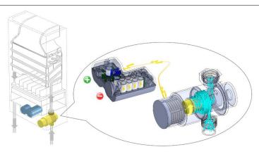
Water Heater Hydropower Generator Module transforms energy generated from water flow into electricity to ignite the appliance, eliminating the need for regular battery replacement in water heaters, thus significantly reducing the environmental pollution arising from the disposal of depleted batteries.
