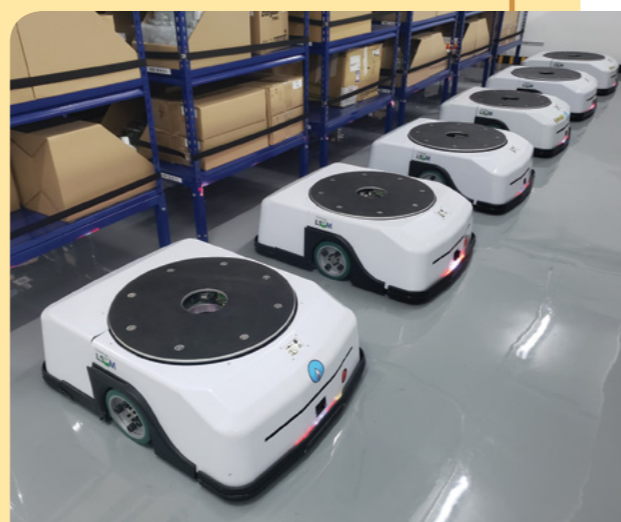
Automated Guided Vehicle In collaboration with the Logistics and Supply Chain MultiTech R&D Centre, we developed this intelligent Automated Guided Vehicle which automates the delivery of shelves to employees.
