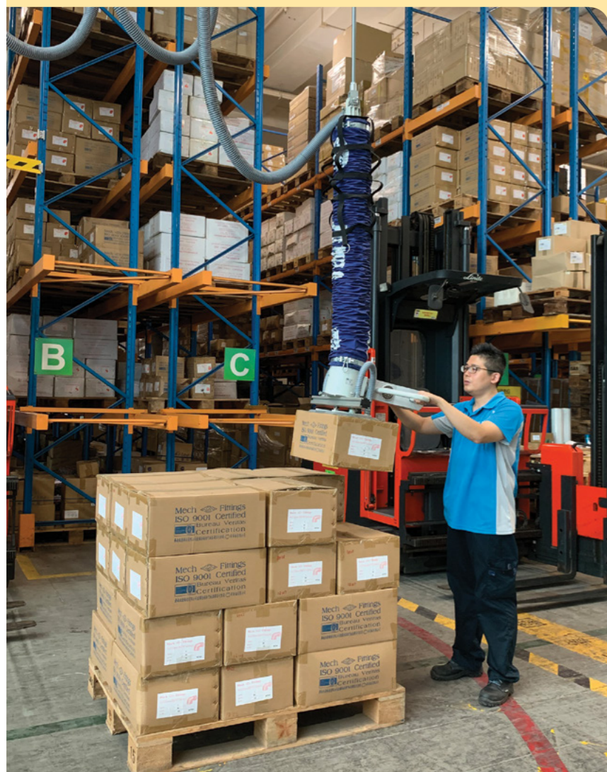
Vacuum Lifter Manual handling work is replaced by this Vacuum Lifter, which applies suction force to lift heavy goods, thus reducing the risk of musculoskeletal problems and related occupational hazards.
