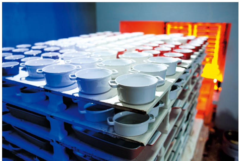
The use of natural gas at this ceramic plant during the firing process not only helps to prevent discolouration, it also improves quality and reduces costs.
