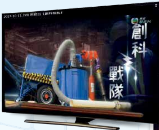
電視台正拍攝「氣動吸泥機」如何有效幫助工人避免長時間彎腰和進行重複性動作。 Pneumatic Soil Remover helps to reduce abnormal posture and repetitive actions of workers.
